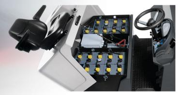
In the B version the box that houses the electrical devices is positioned centrally so it is The opening gives complete accessibility to the components. quick and easy to check the devices and the level of the fluid in the battery elements. A battery box can be installed with a capacity of up to 480 Ah C5 (CS90 B-CS110 B is now very easy.
