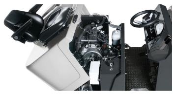
Just the checking of the oil or changing the filters for instance, in the motorised version,
