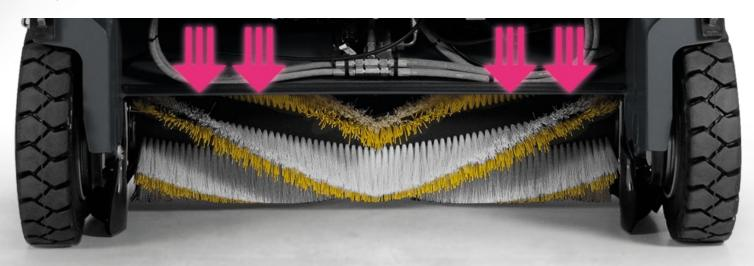
THE CENTRAL BRUSH IS THE FLOATING TYPE AND SELF-ADJUSTS TO KEEP IN CONTACT WITH THE GROUND ALL THE TIME
