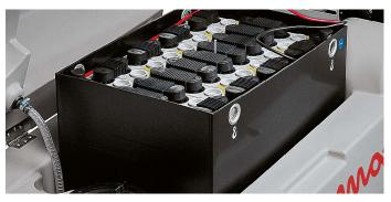
The battery compartment is positioned at the centre of the machine and it is integrated in the tank's volume. All around the batteries, the plastic materials are resistant to oxidising vapours so that any ugly and harmful rust formation is prevented.
