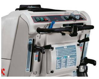
On the machine rear are the controls for lifting and adjusting the scrubbing head as well as the levers for service and parking brakes. There are also two drain plugs on the recovery tank, one being larger for easier internal cleaning.
