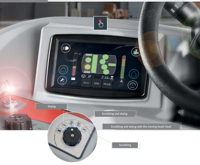
Using the C130 is simple, intuitive and practical. The working program selector enables the operator to manually select the type of activity to be carried out: scrubbing and drying, scrubbing and drying with the moving brush head, scrubbing only, or drying only.
