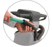
VISPA 35 B-BS Periodic cleaning of the squeegee hose to ensure efficient suction.
