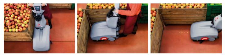
Vispa 35 is ideal for accurate cleaning of room corners and to operate in congested areas thanks to its handle bar which ensures 180° flexibility and to its compact size that is shaped around the brush head.
